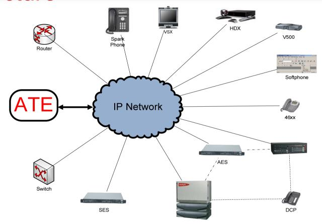
Our Groovy-based Automated Test Environment (ATE) is very complex and includes an extensive set of functionalities for interacting programmatically with our VoIP phones
